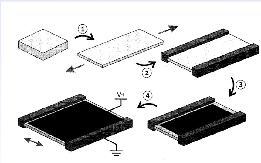
Process of generating pre-strained elastomer film
