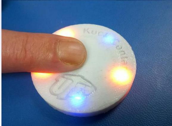
Embedded capacitive sensor in FDM part
