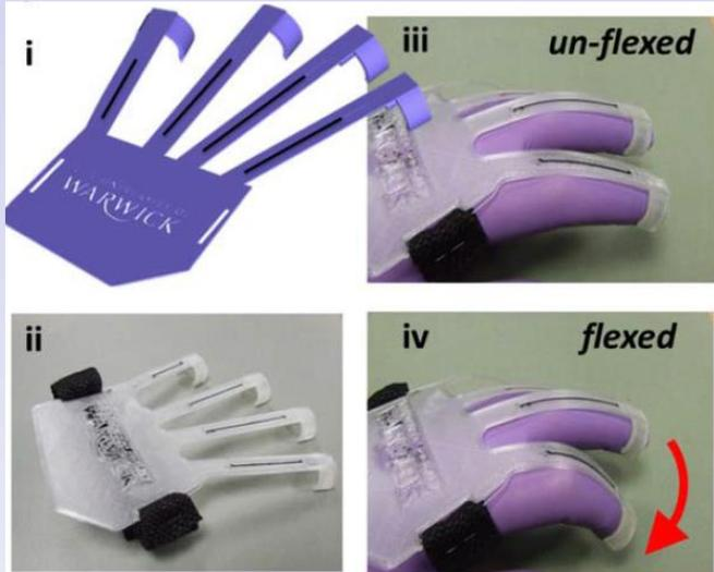
Flex sensor based on piezoresistivity
