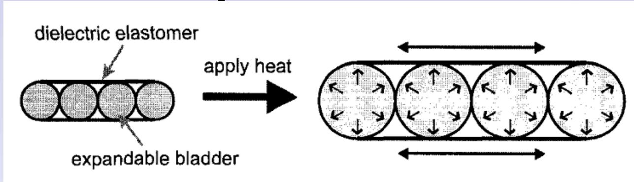
Inflatable structure to generate pre-strain
