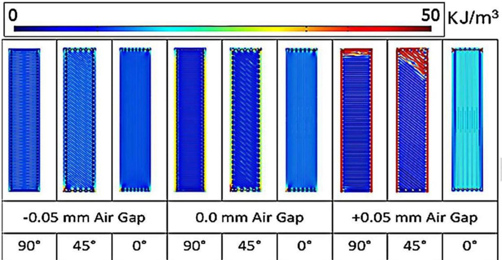
4 Strain energy density distribution in FDM part for different raster angles and air gaps
