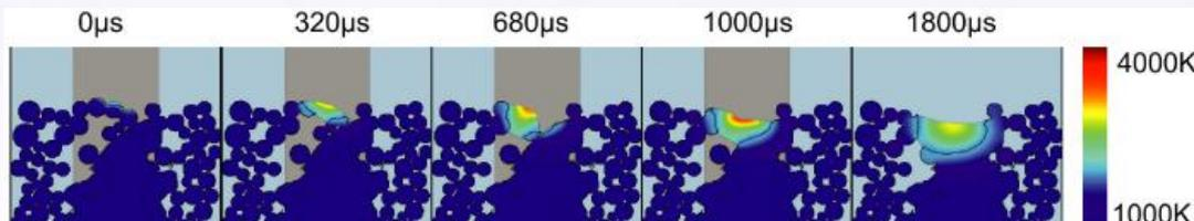
Wetting dynamics: interaction between melts and powder particles
