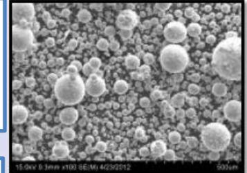
Titanium Alloy (Spherical)
