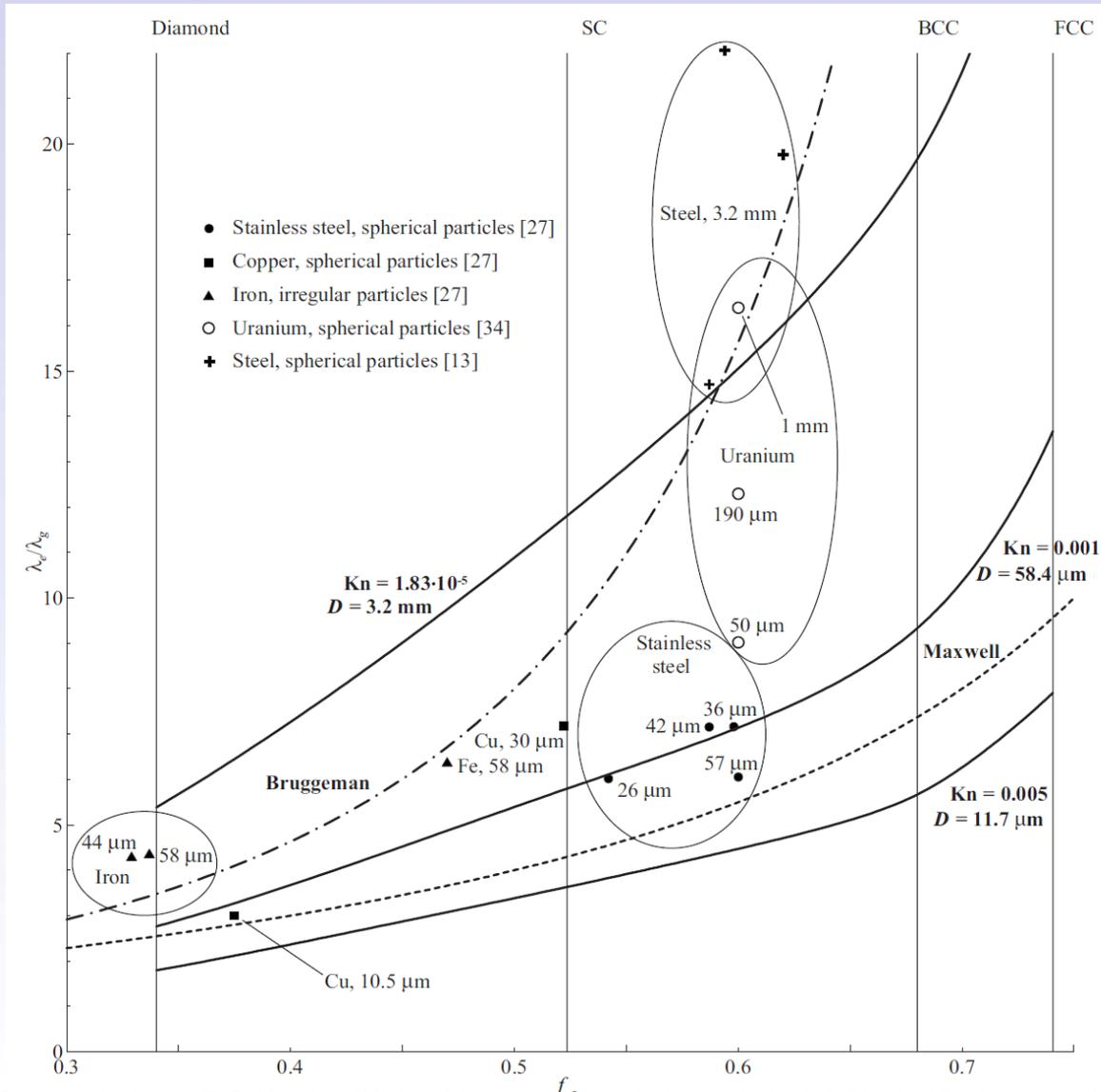
Effective thermal conductivity for different volume fraction (packing)
