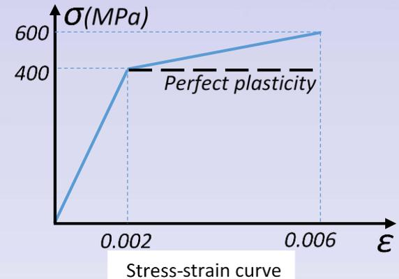
❖ **Case A:** The temperature in the steel bar is uniformly risen from 300 to 1,100 K and then cooled back down to 300 K. Will there be any residual stress in the bar?
