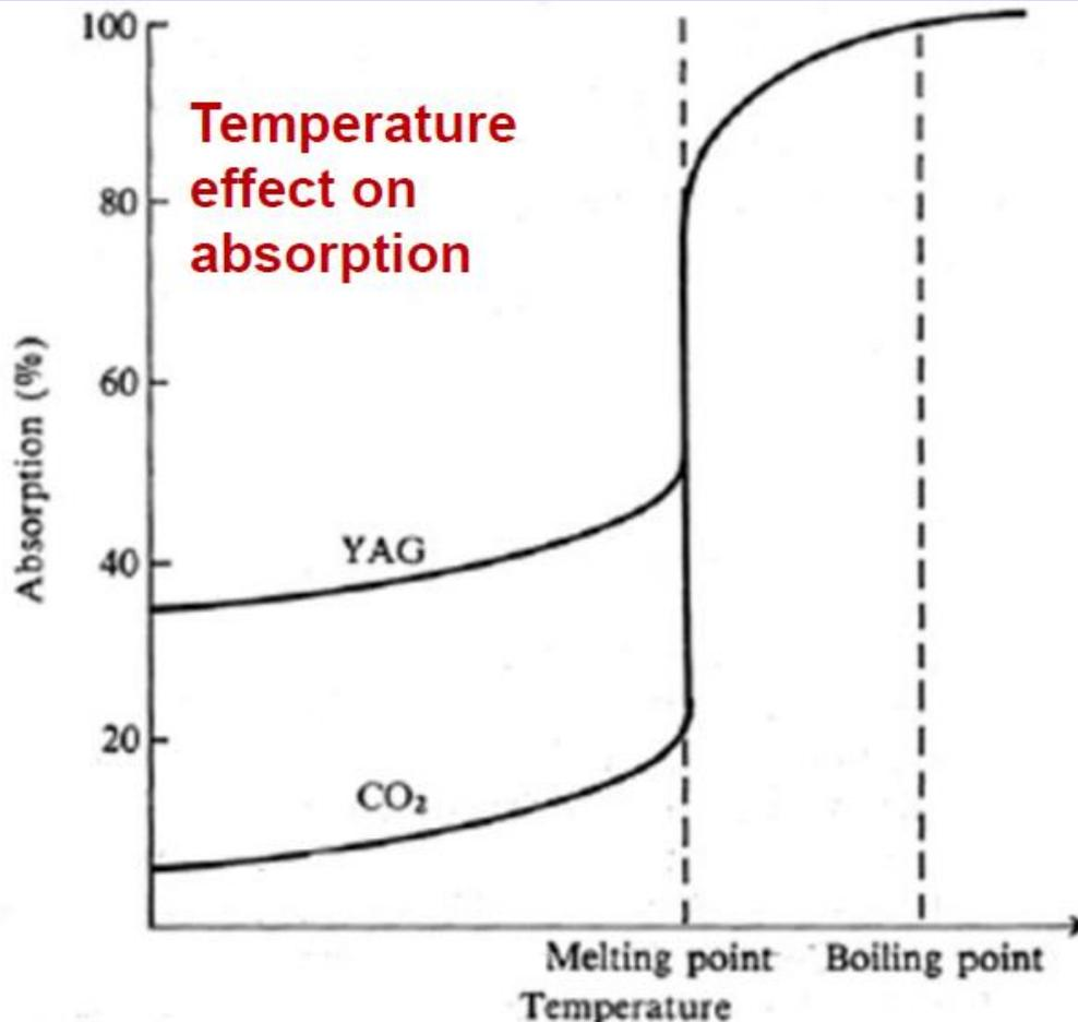
❖ **Absorption and reflectivity are very temperature dependent, often undergo significant changes when material melts, e.g., silicon, steel becomes highly reflective on melting**
