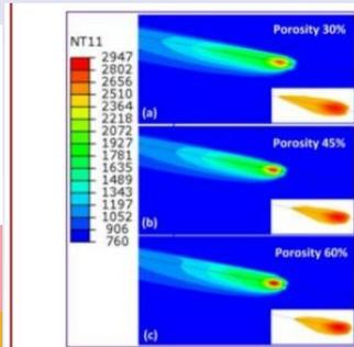
Fig. 13 Temperature fields and molten pool geometries of powder bed of various levels of porosity
