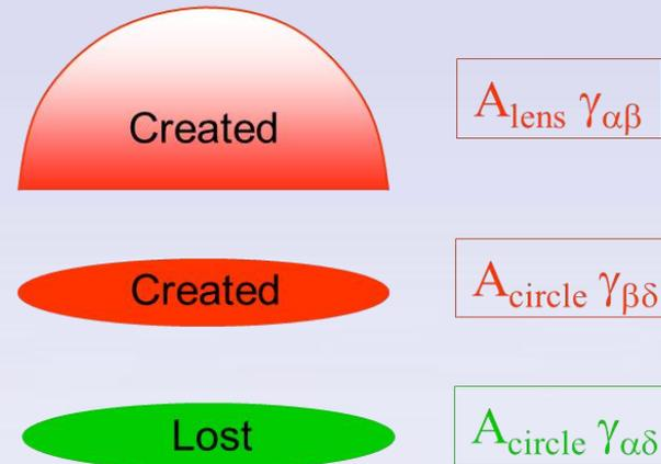
Surface tension force balance  $\longrightarrow \gamma_{\alpha\beta} \text{Cos}\theta + \gamma_{\beta\delta} = \gamma_{\alpha\delta}$
