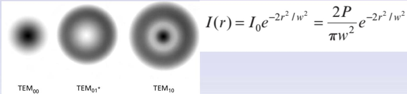
Traverse mode: Gaussian beam (lowest order mode), need mode control
