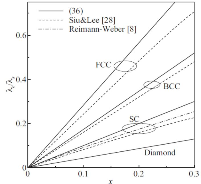
Effective thermal conductivity VS different contact size
