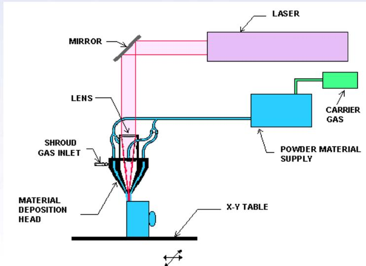
Laser Engineered Net Shaping /Direct Metal Deposition
