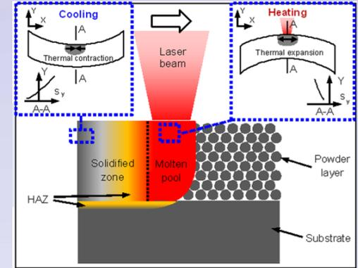
Thermal expansion and internal stress
