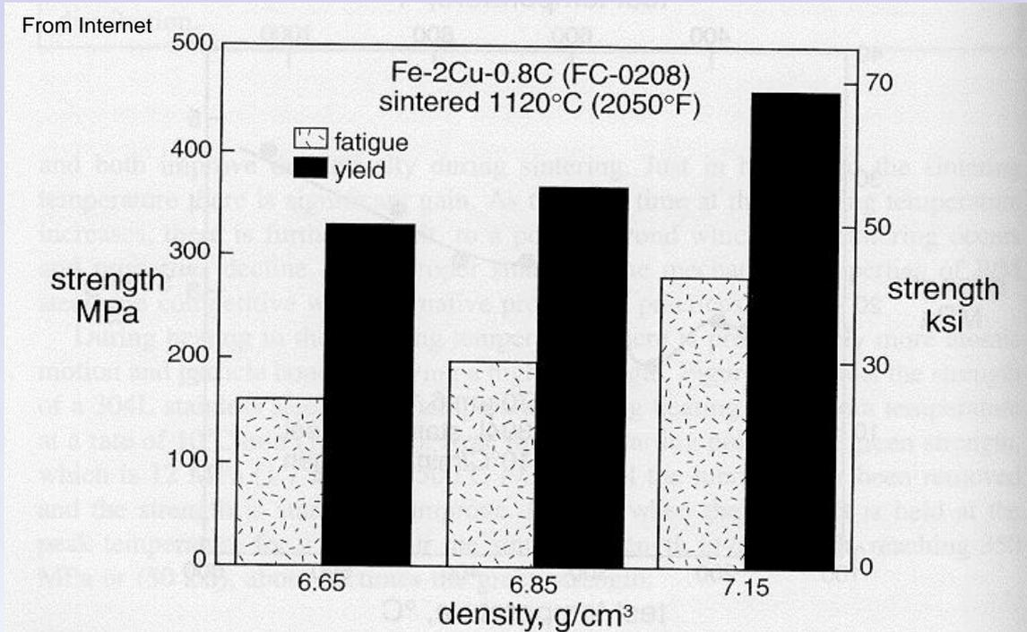
**Figure 6.23.** Yield and fatigue strength of sintered Fe-2Cu-0.8C (FC-0208) shown as a function of the green density, for a constant sintering cycle of 1120°C (2050°F) for 25 min. (Data from Kevin Christian.)
