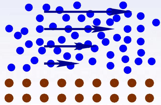
**No-Slip Boundary Condition breakdown near the wall**
