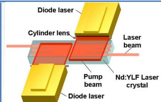
Diode-pumped solid-state laser
