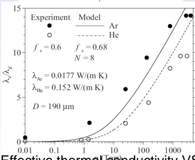
Effective thermal conductivity VS different gas pressure
