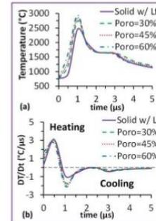
Fig. 14 Temperature histories and heating or cooling rates of center point for various levels of porosity
