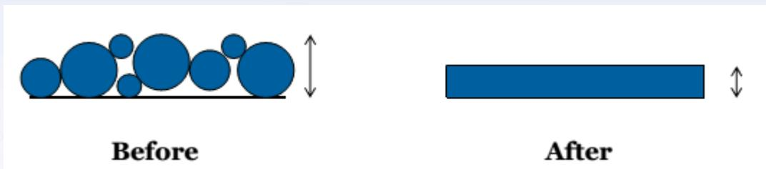
Affecting coating thickness: typically thickness before sintering is 2 – 3X of after sintering
