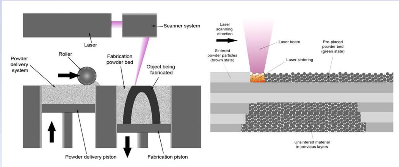
Selective Laser Sintering/Melting, Electron Beam Melting
