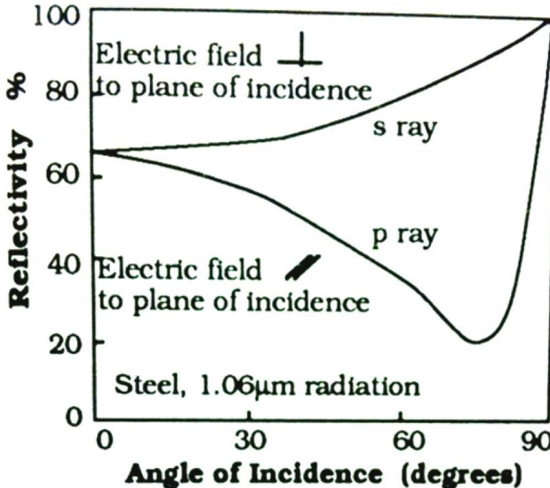
Reflectivity of steel to polarised 1.06 micron radiation
